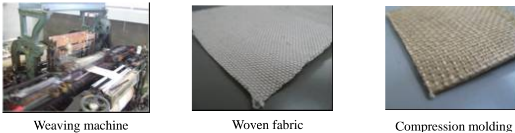
Fig.6 Fabrication of woven fabric composite.
